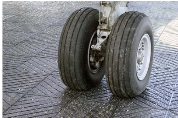
Landing gear on an Endura-Form panel deck.
