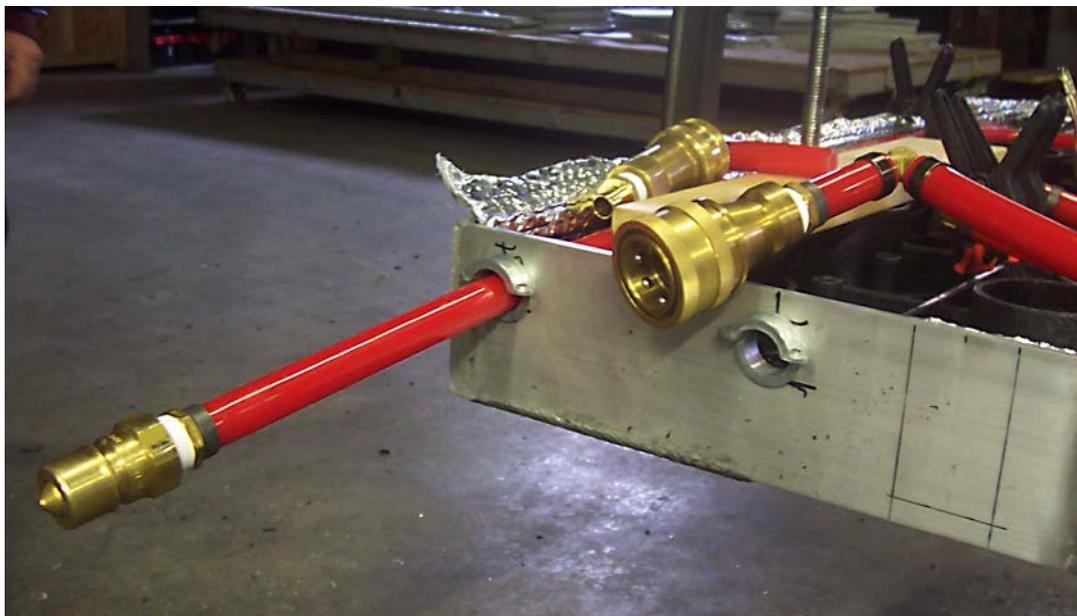
**Figure 11:** This shows the male and female quick connectors. The right hand line has not yet been run through it's port. The quick connectors would attach to the external heat lines which would carry the glycol heating fluid to and from the heating source. The heating source will vary from application to application.
