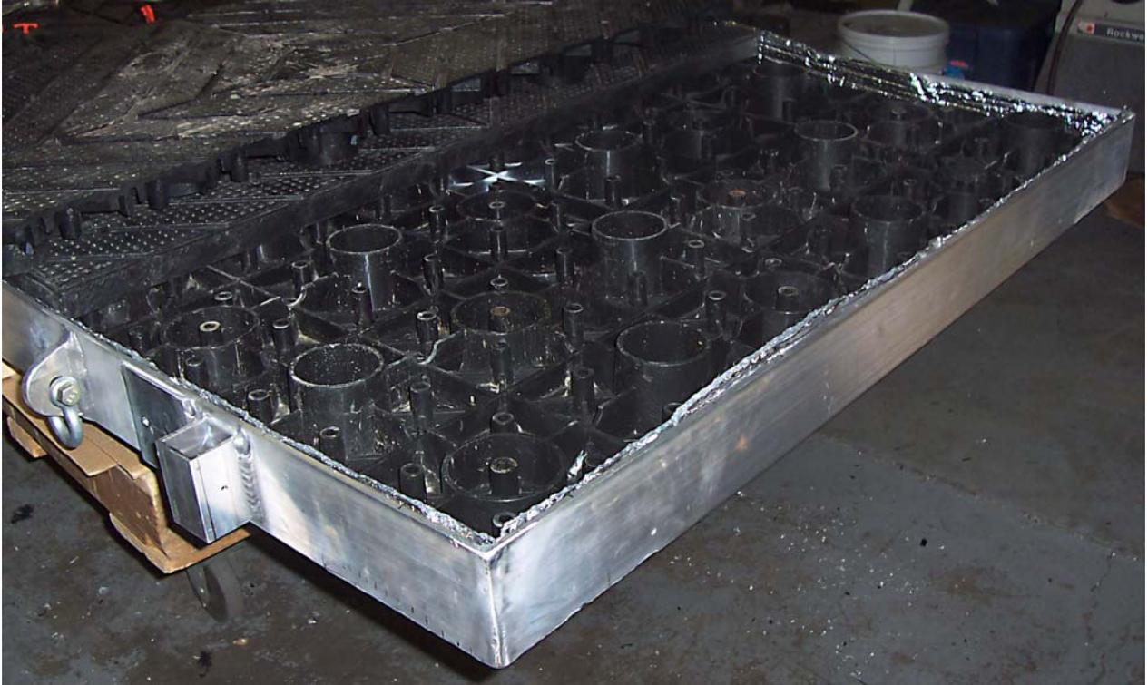
**Figure 13:** This shows the upper Endura-Form panels being fitted. The panels are fitted in an offset pattern to allow for interlocking thus making them a virtual continuous assembly. In this example the heating lines are not fitted. The top layer is fastened with bolts that thread into fixed receiving nuts in the bottom layer making for a very strong panel group. The modular nature of the panels makes it easy to replace damaged panels or to provide access to the heating lines.
