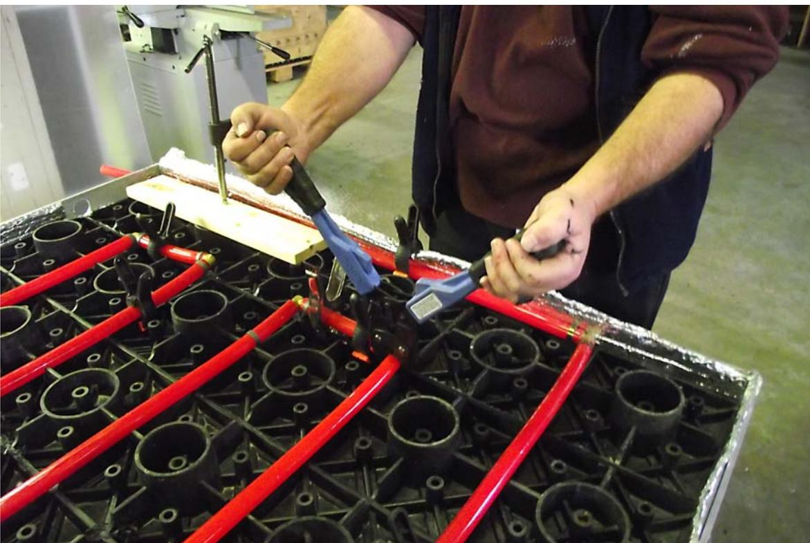
**Figure 09:** This shows the heating lines being crimped to the fittings with a special crimping tool. At the upper left can be seen the ports for the inflow and outflow lines. The inflow and outflow lines can be put in different places.
