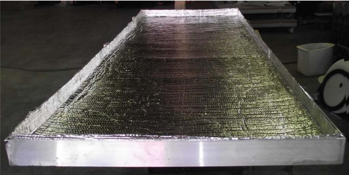
**Figure 04:** The assembled aluminum tray is lined with insulating material to minimize heat loss through the aluminum and maximize the heat traveling to the surface. The insulation is cut to allow for the drain holes.
