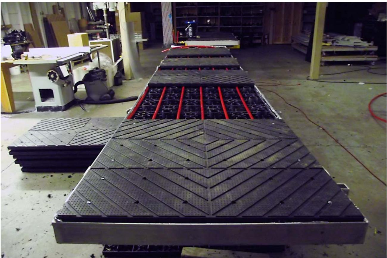
**Figure 14:** This shows the top layer partially assembled - you can see the half panel at the near end that gives the panels their interlocking offset. A few bolts are also in place.
