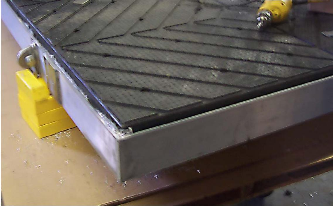
**Figure 15:** A closer look at a corner of the walkway with the upper Endura-Form panels in place but not yet bolted. The Endura-Form panel surface is grooved for maximum drainage and has a dimpled surface to allow for good traction. The Endura-Form panel assembly is held in place in the aluminum tray with tabs placed at appropriate intervals. A yellow walkway stand is visible on the left.
