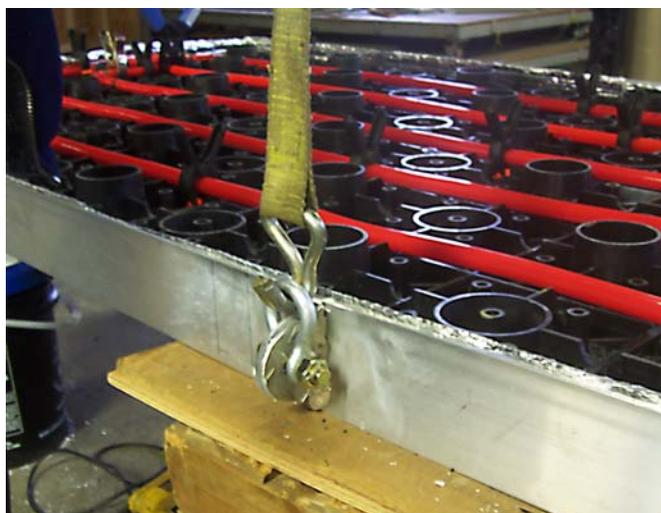
**Figure 12:** This shows one of the lifting lugs and shackle with a hook and strap ready to be lifted.
