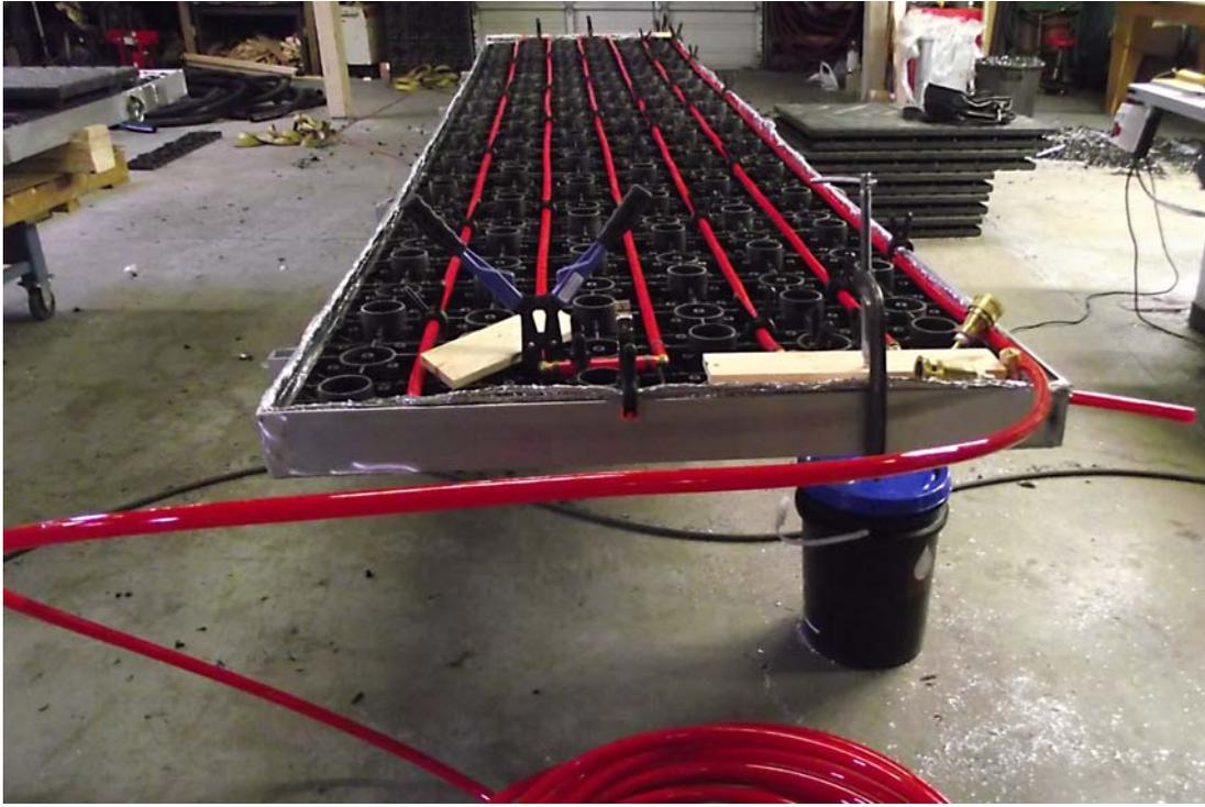
**Figure 10:** This shows all six heating lines in place. The near right corner has the inflow and outflow lines which are not yet completed.
