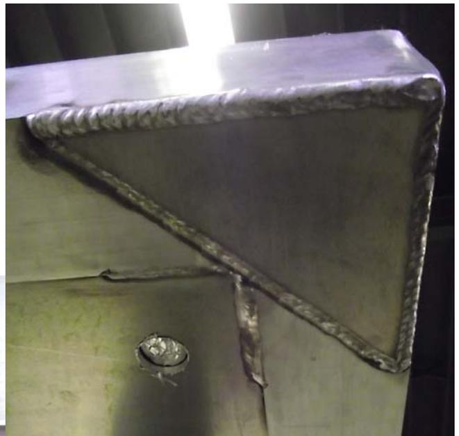
**Figure 03:** This view shows the 1/4" aluminum reinforcing at each corner for maximum strength. A drain hole is also visible - the drain holes are 1 3/8" diameter.
