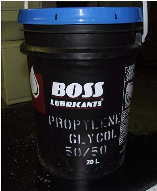
**Figure 18:** The heating liquid is food grade propylene glycol. The walk shown would take approximately 3 gallons, not including the outboard connecting lines. Over 4 hours the glycol should reach a temperature of 170° F. Over six hours a temperature of 185° to 190° F.
