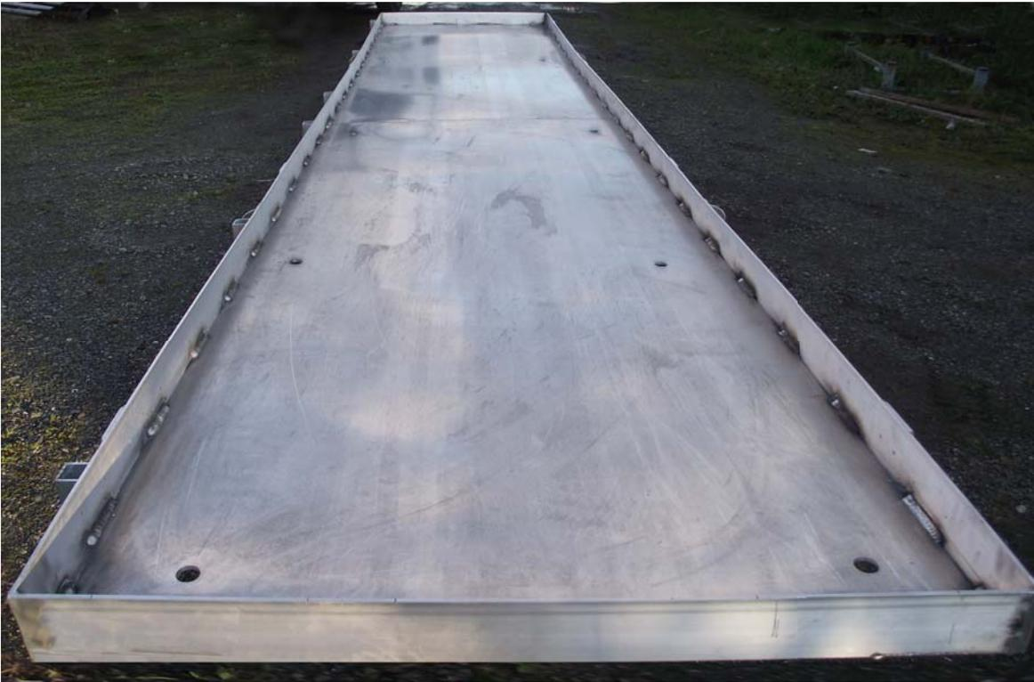
**Figure 01:** This shows the assembled aluminum tray that will hold the Endura-Form panel assembly. This framework gives the assembly great rigidity and strength allowing it to be easily handled and it can be placed on blocks or stands if needed. The 4" x 4" x 1/4" aluminum angle with a 1/4" aluminum sheet is welded to the bottom. Drain holes are fitted at regular intervals to allow melt water to drain away. The solid bottom also gives protection from any surface the walkway may rest on.
