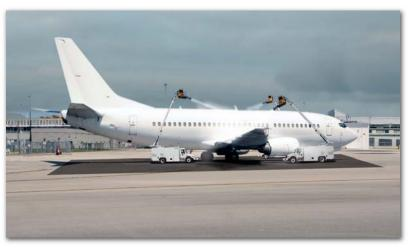
a sump from where it can be pumped to a containment unit - no more puddles of deicer fluid building up and none getting into the storm drains. The decks can easily be made any size to accomodate any aircraft and installed either level to the parking apron or on top of it with a suitable ramp for easy access. Endura-Form panels can also be fitted with radiant heat systems to keep the decks clear in the toughest weather.
