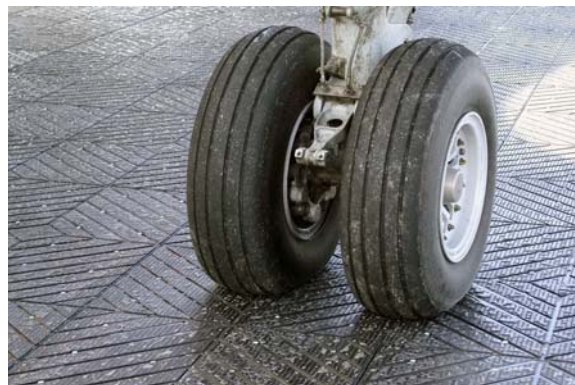
Landing gear on an Endura-Form panel deck.
